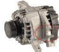
Broken fixing hole
